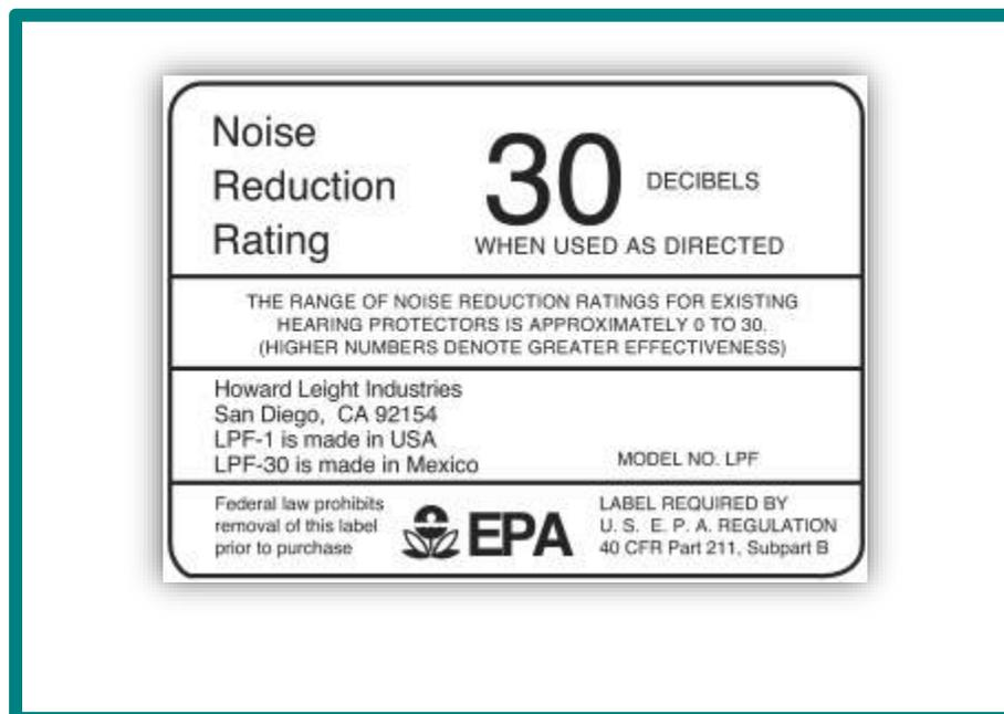
The NRR describes the average sound level reduction (attenuation) provided by a hearing protection device (HPD) in a laboratory test. Since the NRR is based on laboratory testing, it does not take into account the loss of protection that occurs
